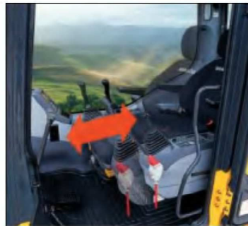
Seat Sliding Amount: 340 mm 13.4", increased 120 mm 4.7"
